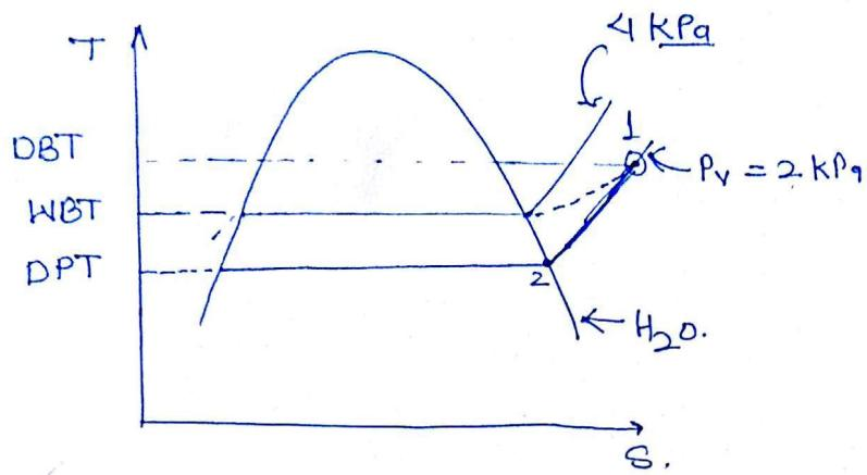
$\left\{ \begin{array}{l} \text{unsaturated} : \quad DBT > WBT > DPT \\ \text{saturated} : \quad DBT = WBT = DPT \end{array} \right.$
