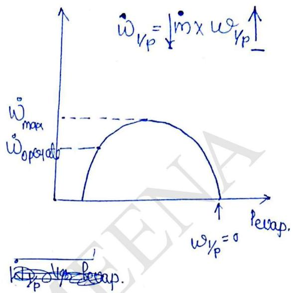
\* The operating is less than the maximum bar power but the compressor motors are designed for maximum power conditions because for reaching the operating power we have to cross the max. power condition.
