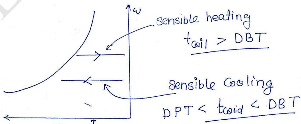
The process followed in the electrical room heater is sensible heating
