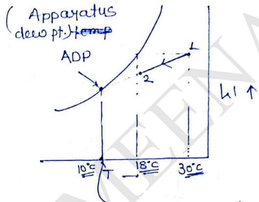
⇒ The cooling and dehumidification lines when produced intersects the saturation curve at the point called as apparatus dew point. The temp. corresponding to this point is the temp of the cooling coil. called as apparatus dew point temp
