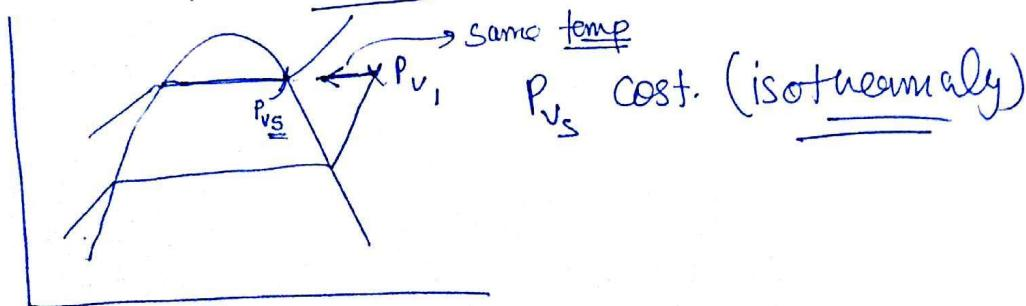
P Moist air at a pressure of 100 kPa is compressed to 500 kPa and then cooled to 35°C in a cooler at const. pressure (there is no condensation). The air at the entry to the cooler is unsaturated and becomes just saturated at the exit of cooler. The saturation pressure of vapour at 35°C is 5.628 kPa, find partial pressure of vapour in moist air entering the compressor.
