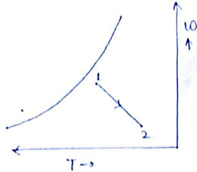
This process is carried out with the help of chemicals like alumina ( $\text{Al}_2\text{O}_3$ ). These chemicals absorb water vapour from the air and ~~water~~ water vapour while leaving the air, condenses and reject latent heat of condensation in the air, hence the temp of air increases.
